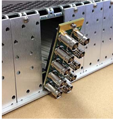
Figure 4. Rear Card Inserted Into Frame Seating Slot
